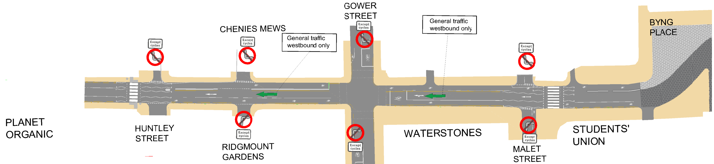
Drawing 2: Torrington Place to Tavistock Place westbound option without stepped cycle tracks & pavement widening
